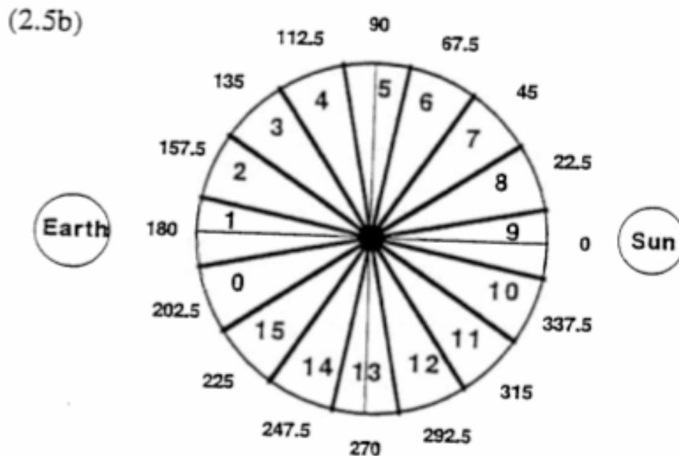
Figure 2. STICS spins through 360 degrees during one measurement cycle sweeping out 16 sectors in space. Sectors 8-10 include the solar direction (Adapted from Chotoo et al. 1998).
